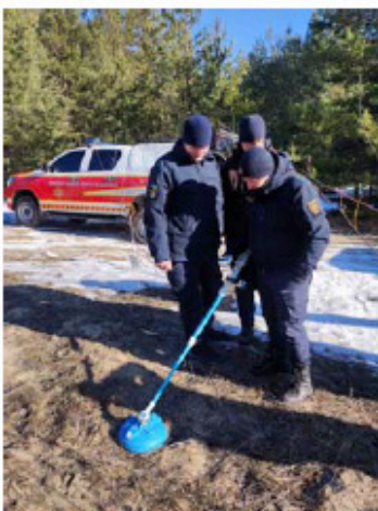
Figure 1: Mine detection by GPR in Ukraine
